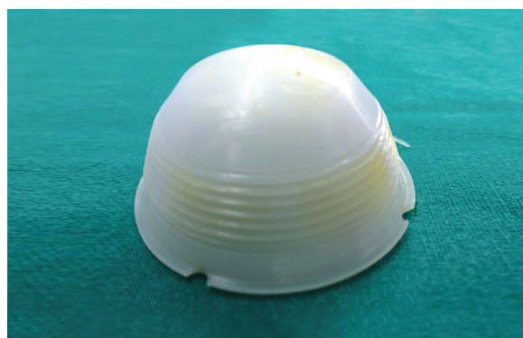
Figure 5: The back of the liner does not show wear out of locking mechanism. A small piece on the right of the liner comes from the extraction procedure.
