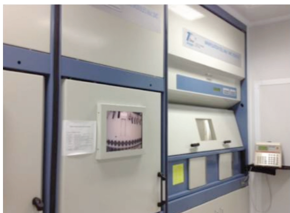
Figure 3: Hot cells and a manipulation hot cell situated in a controlled clean room
